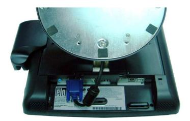
• Connect one end of the **video cable** to the rear side of computer and the other to the LCD monitor. Tighten by turning the two thumb screws clockwise to ensure proper grounding.
